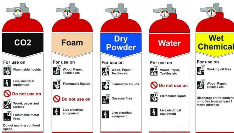
Fig. 7.2.4 Types of Fire Extinguishers
