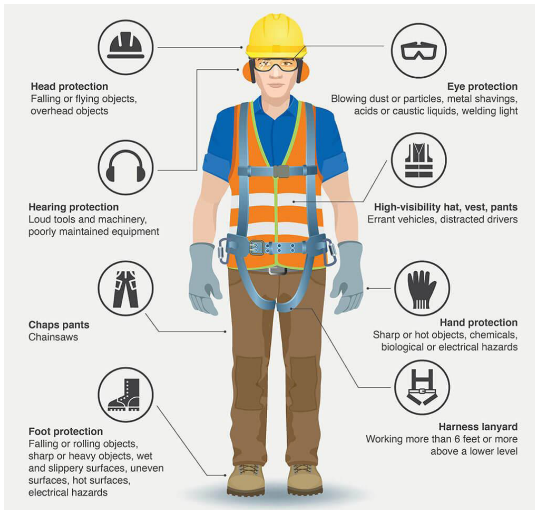
Fig. 7.2.16 A Construction Worker with proper PPEs
