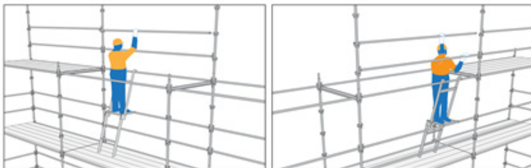
Fig. 2.2.7 Dismantling of scaffolding
