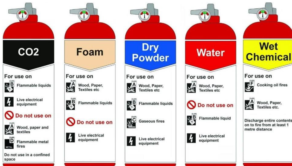
Fig. 5.2.4 Types of Fire Extinguishers
