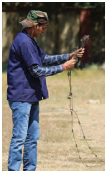
Fig. 3.2.5 Folding the chain
