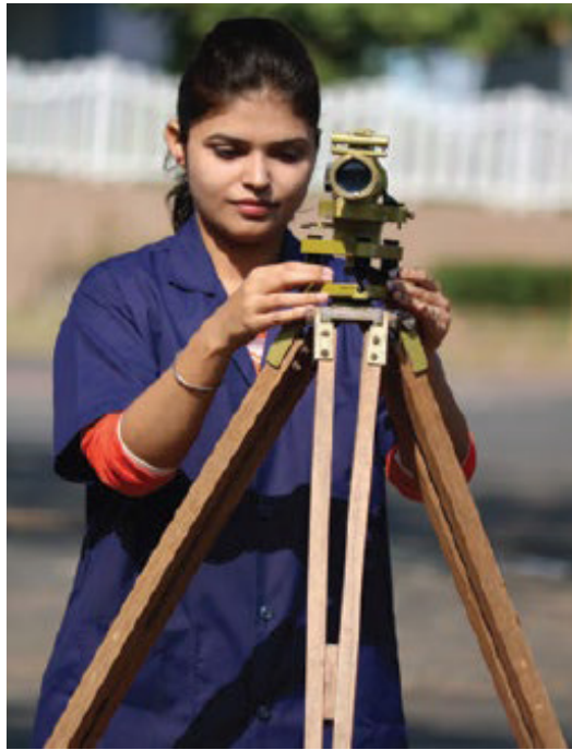
Fig. 3.1.6 Placing over the located point and adjusting the instrument.
