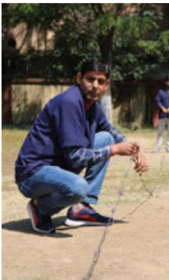
Fig. 3.2.4 Stretching the chain in line
