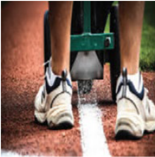
Fig. 3.3.8 Lime Application over the String Line using Lime Applicator
