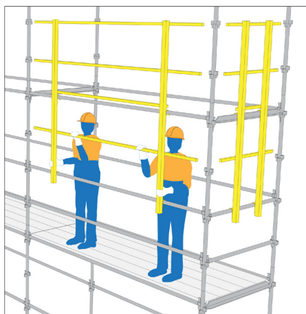
Fig. 3.1.2 Erecting and dismantling temporary scaffolding
