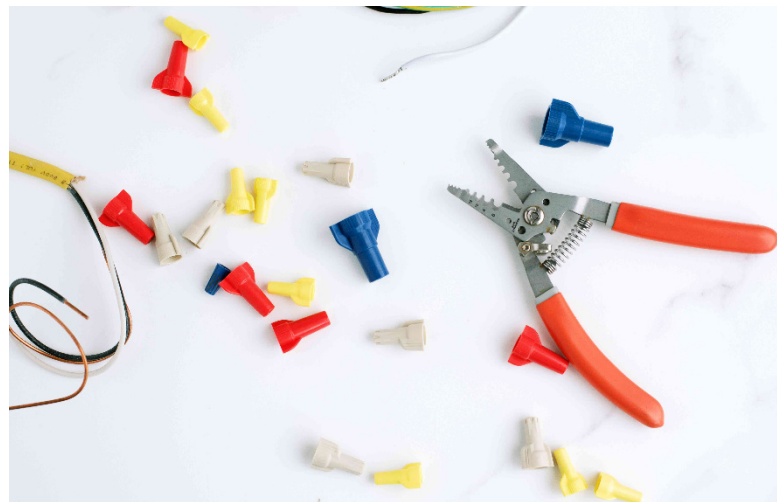
Fig. 4.1.23: Termination of electrical wires/cables by wire nuts
