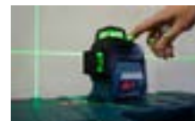
Fig. 2.1.9 Laser Level (Source: https://www.911metallurgist.com/blog/laser-levels/ )
