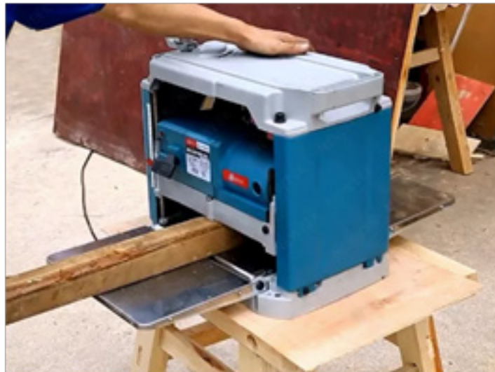
Fig. 3.1.14 Planing Machine used for Planing Shutter Boards
