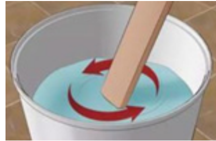
Fig 4.1.8 Mixing paint and thinner
