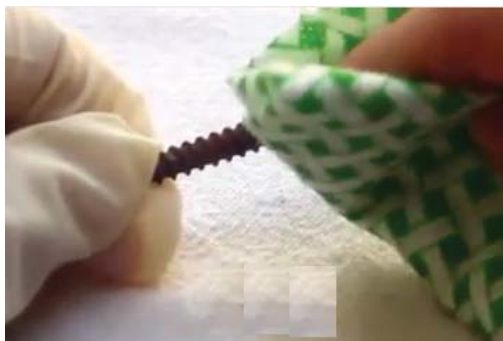
Fig 5.1.3 Cleaning rusty metal surface
