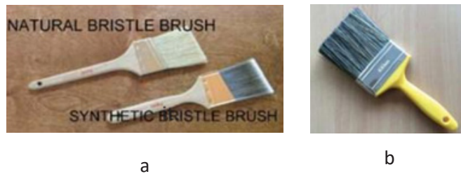
Fig 3.1.2 Types of Brushes: a) Synthetic and Natural Bristle Brush b) Combined Synthetic & Natural Bristle Brush
