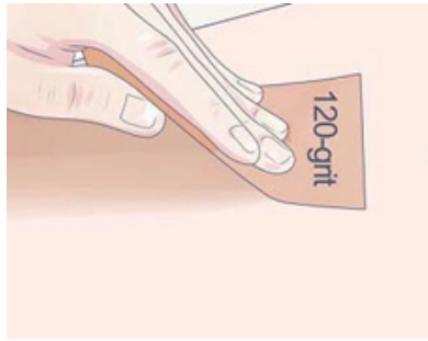
Fig 6.1.15 Sanding of surface
