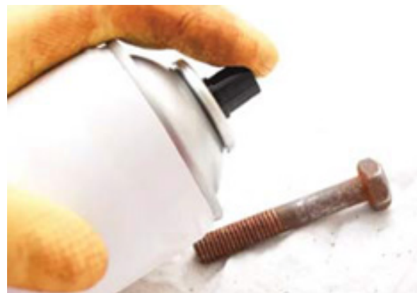
Fig 5.1.6 Priming of metal surface
