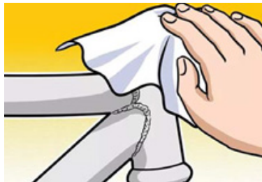
Fig 5.1.2 Cleaning metal surface
