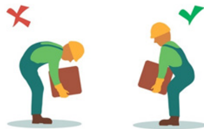
Fig. 3.3.16 Lifting in a right way
