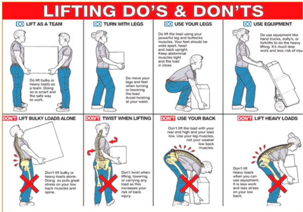
Fig. 3.3.17 Do's and don'ts while loading and unloading the material
