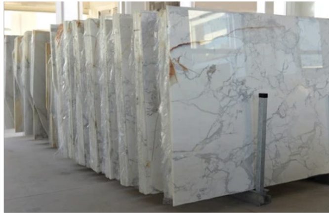
Fig. 3.3.11 Stacking of marble slab
