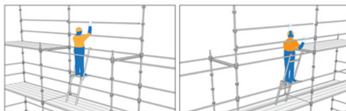
Fig. 5.2.7 Dismantling of scaffolding
