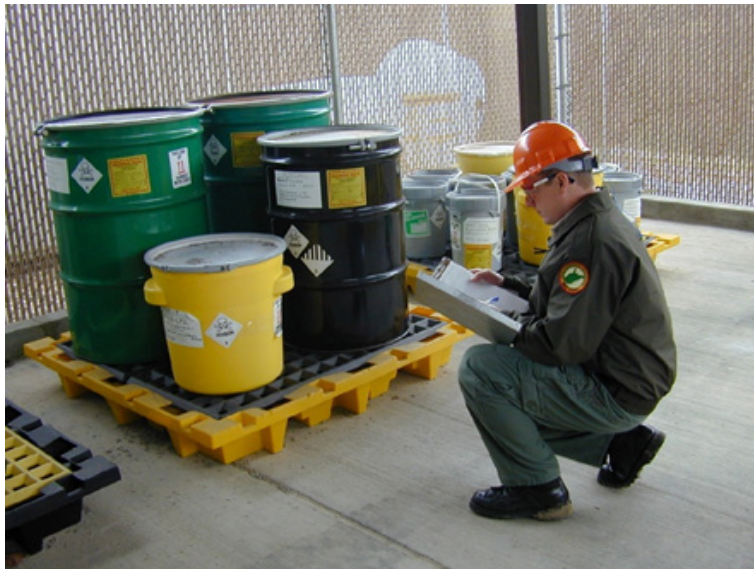
Fig. 3.3.15 Storage of hazardous materials
