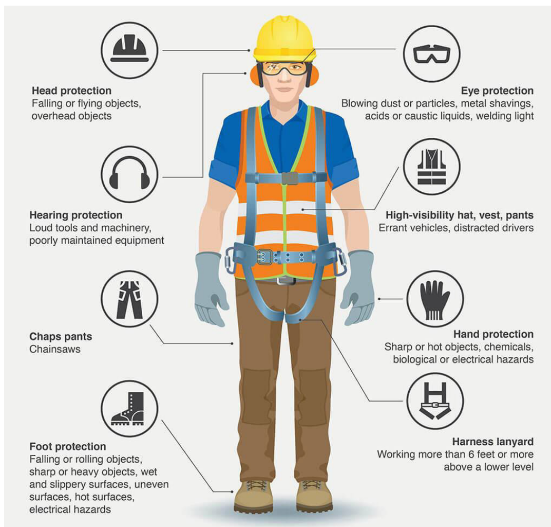
Fig. 7.2.16 A Construction Worker with proper PPEs
