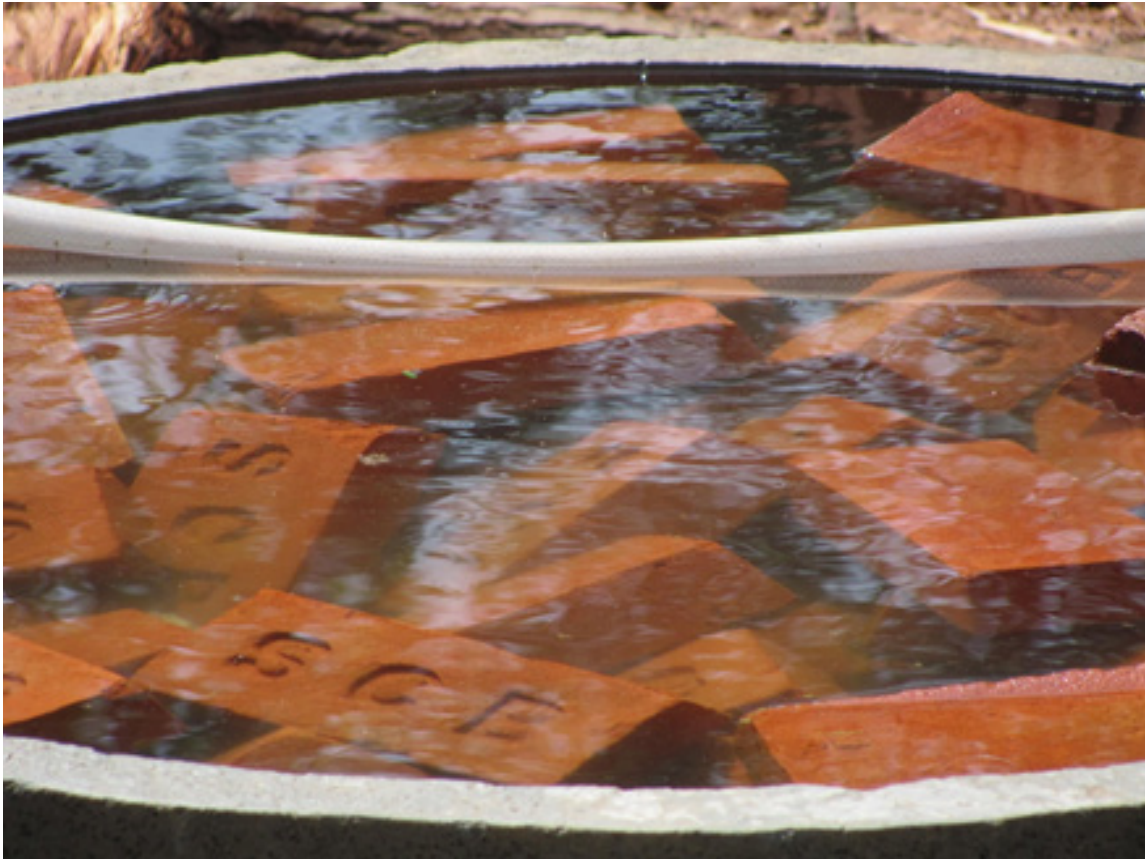
Fig. 6.1.10 Soaking of brick/block
