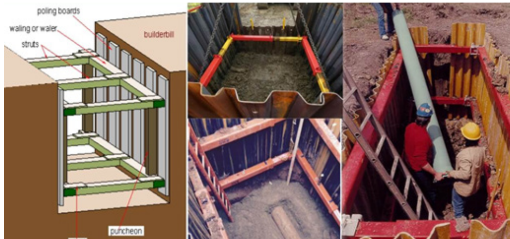
Fig. 4.1.13 Shoring and timbering
