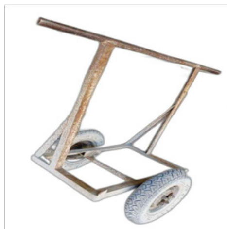
Fig. 3.3.14 Lifting of slab using trolley
