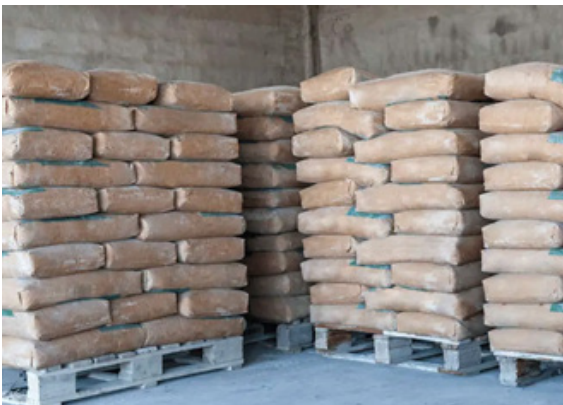
Fig. 3.1.6 Right way of stacking Cement
