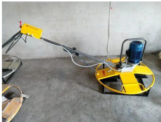
Fig. 4.3.2 Power tools for Tremix Flooring
