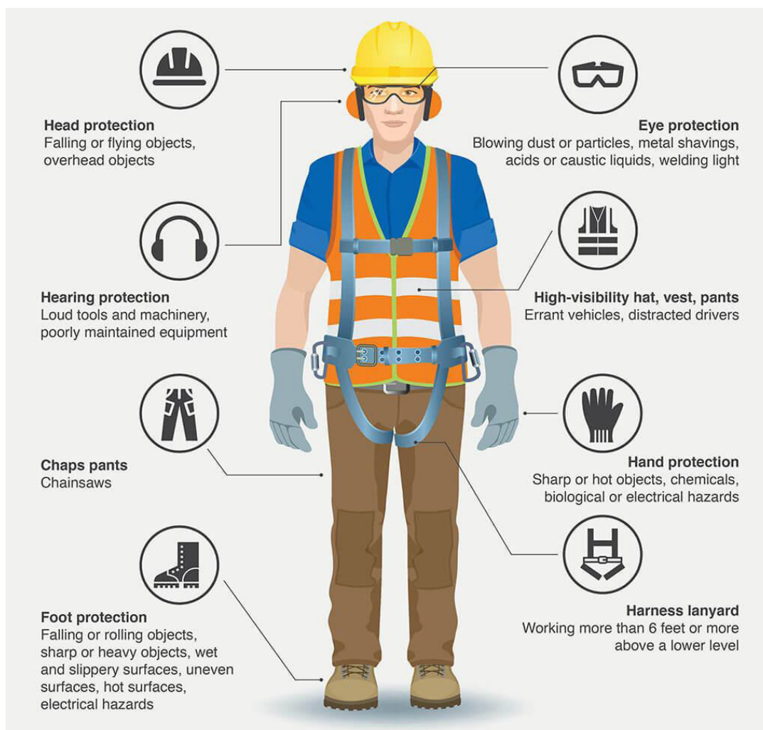
Fig. 7.2.16 A Construction Worker with proper PPEs
