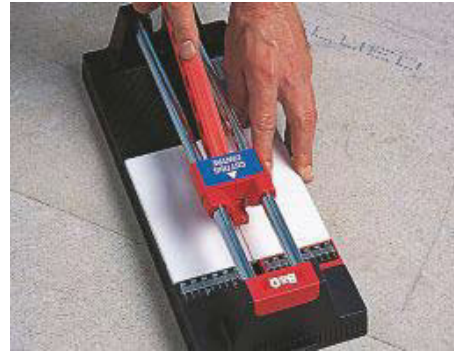
Fig. 4.2.8: Inserting tile in the machine
