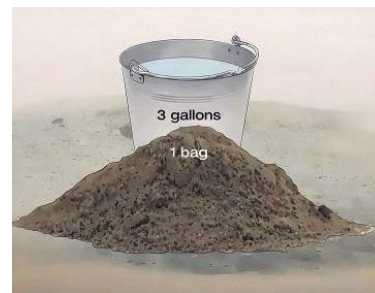
Fig. 4.3.6: Mixing of mortar and water
