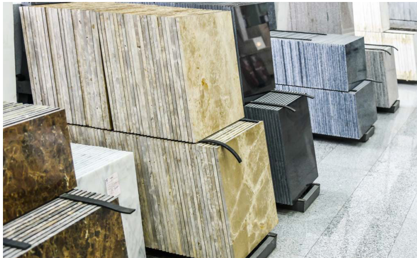
Fig. 3.2.14: Storing and stacking of tiles
