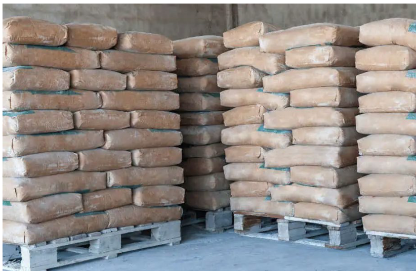
Fig. 3.2.13: Storing and stacking cement or grout bags
