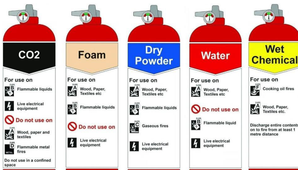
Fig. 8.2.4 Types of Fire Extinguishers
