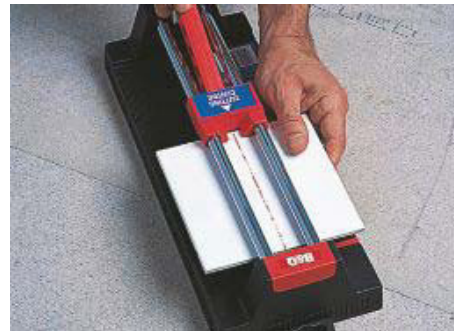
Fig. 4.2.9: Fitting tile in the machine
