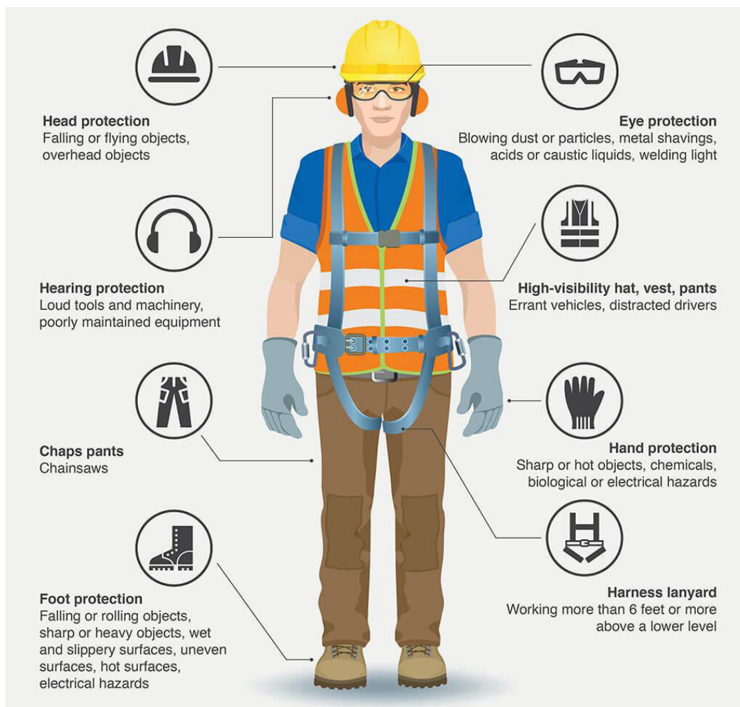
Fig. 7.2.16 A Construction Worker with proper PPEs
