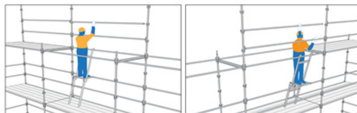
Fig. 6.2.7 Dismantling of scaffolding
