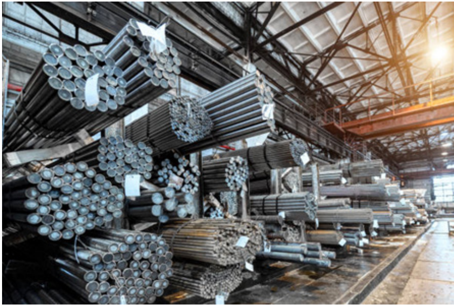
Fig. 3.2.2 Bars stored on wooden beams or platforms to avoid rusting
