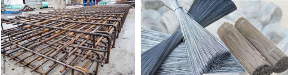
Fig. 3.1.27 Reinforcement bars and binding wires
