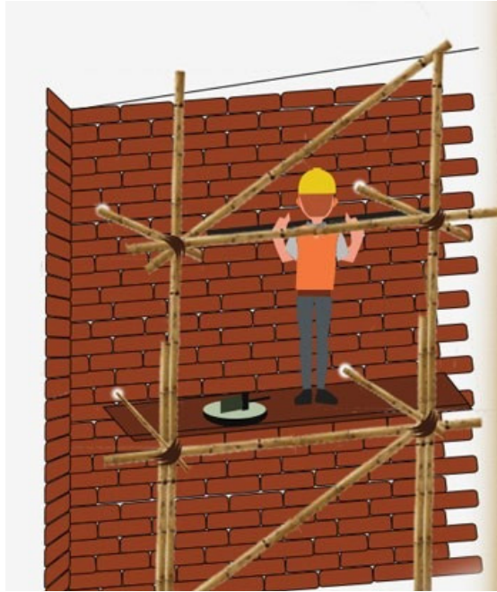
Fig. 6.2.8 Working on bamboo scaffolding
