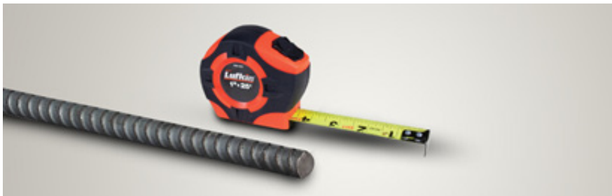
Fig. 5.1.2 Measuring and marking cut lengths
