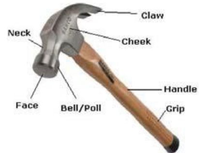
Fig 3.1.12: Hammer and its parts
