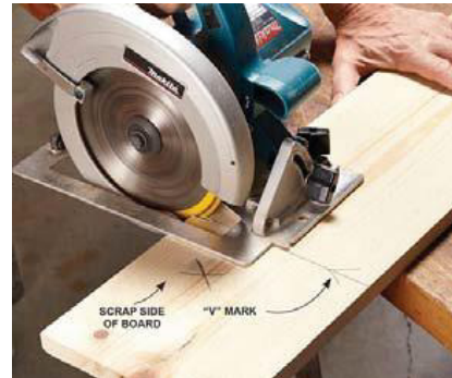
Fig 3.1.23: Use of circular saw
