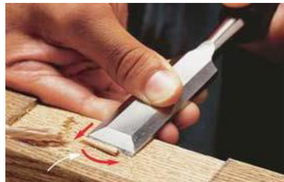
Fig 3.1.9: Paring cut using chisel
