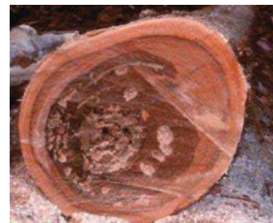
Fig 3.4.13: Defects due to natural force
