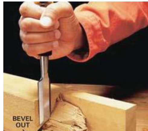
Fig 3.1.10: Chopping cut using chisel
