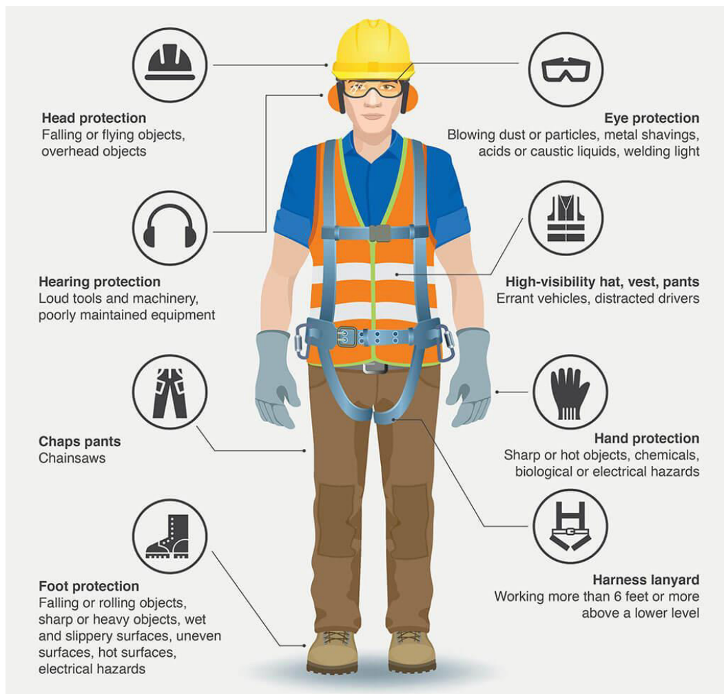
Fig. 7.2.16 A Construction Worker with proper PPEs
