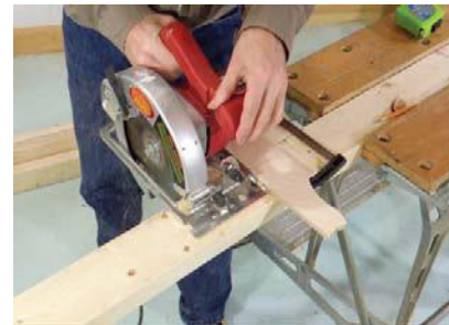
Fig 3.1.23: Use of circular saw
