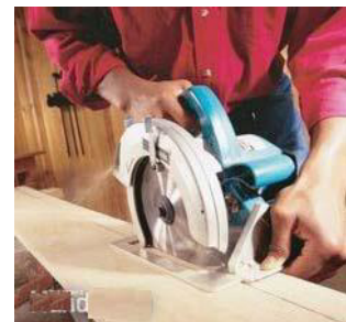
Fig 3.1.22: Use of circular saw
