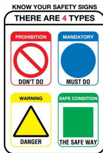
Fig. 7.1.6 Workplace Warning Signs
