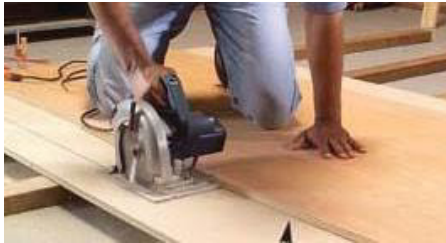
Fig 3.4.22: Cutting wood by circular saw
