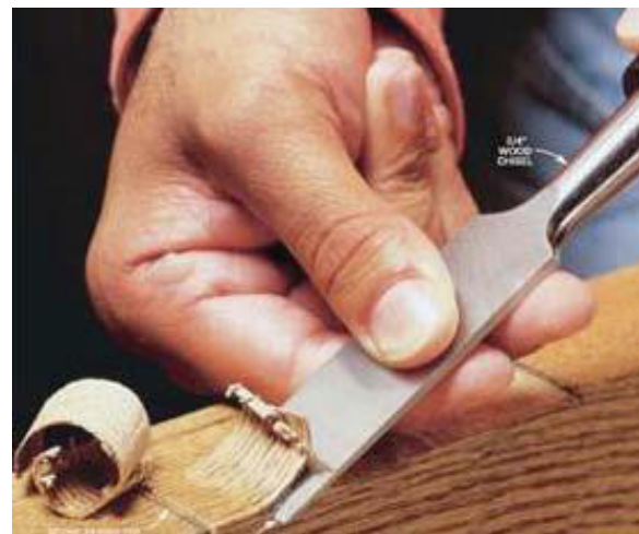
Fig 3.1.8: Mosaic cut using chisel
